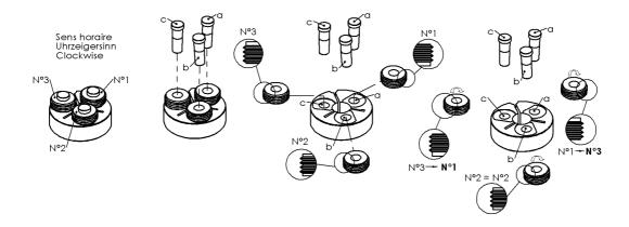
Assembly of the roll No 2, moving and assembling the rolls No 1 and No 3
