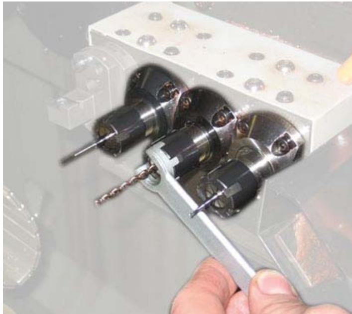
**In this picture you can see a typical example of a 3-spindle head from a Swiss turning lathe with standard ER-Mini collet nuts.**
